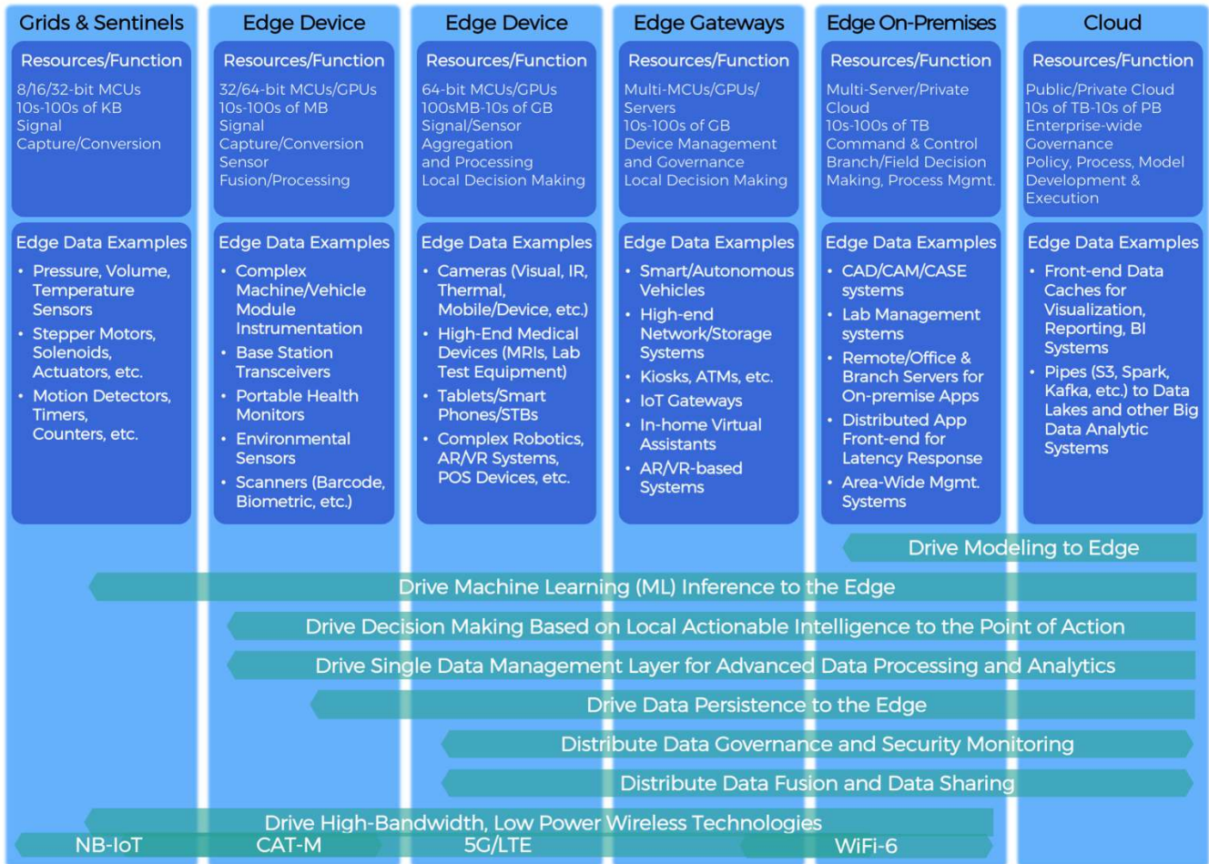
Figure 4: Where Edge Data Management is Required and Changing Demands on how and where it's needed.
