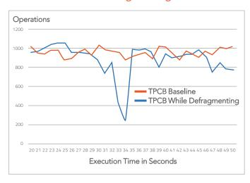
Reads and writes continue uninterrupted during defragmenting, which runs at lower priority than normal operations. The following chart compares a standard TPCB benchmark test with and without Defragmenter execution.
